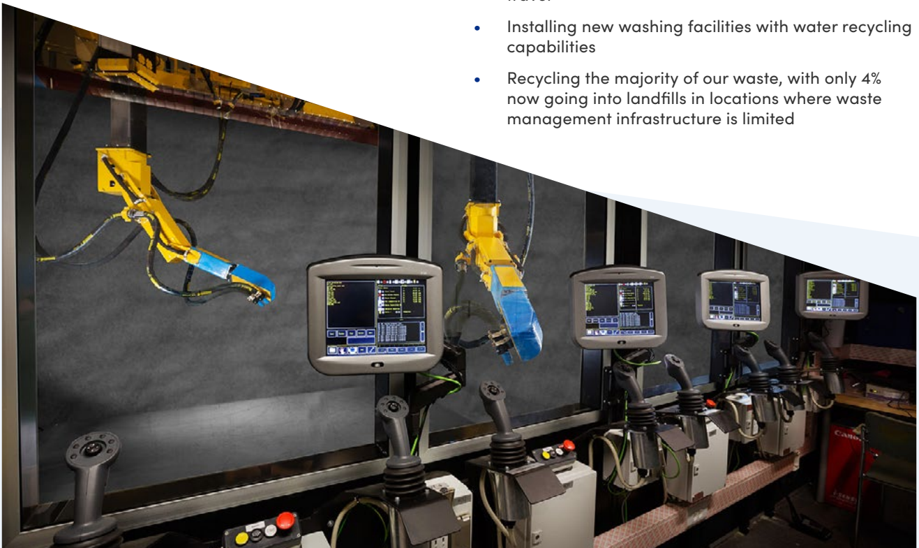
A multi-million-pound investment in robotic blast and paint coating technology to drive progress toward our net-zero target.
