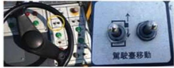
Install dual control switch for movement of operator's panel or bridge platform of main and lower deck loaders
