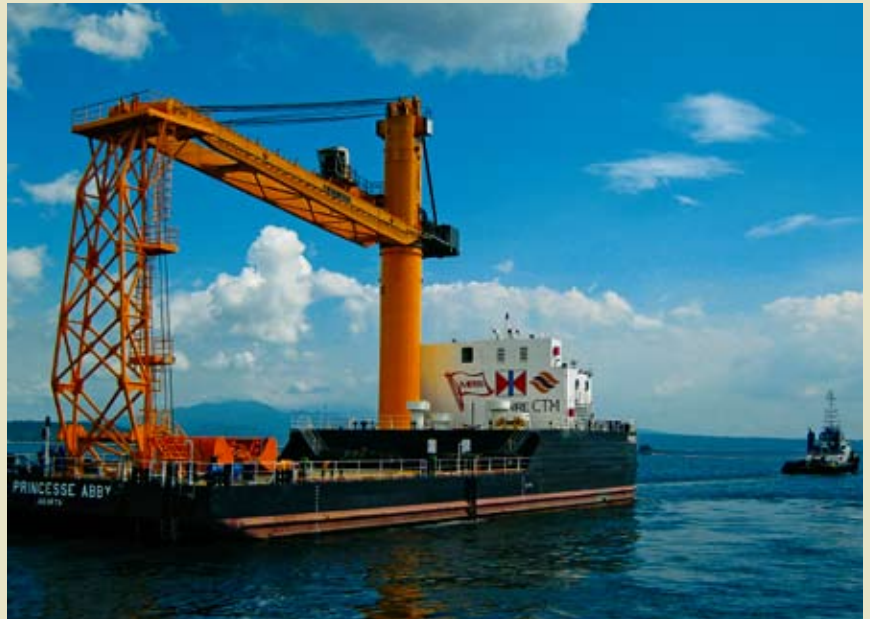
Princesse Abby, the newly launched floating crane belonging to recently established China Navigation Company joint venture Swire CTM Bulk Logistics, at work transshipping coal off Kalimantan in Indonesia, where she is on charter to local Indonesian partner, PT Mitra.
