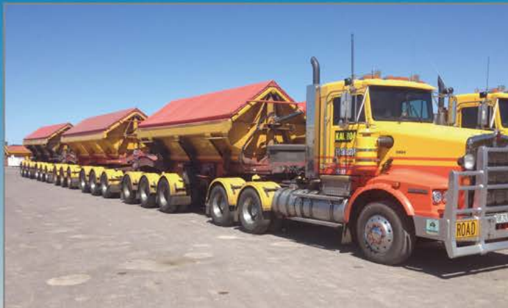
A triple road train can take up to 500 metres to stop when fully loaded
