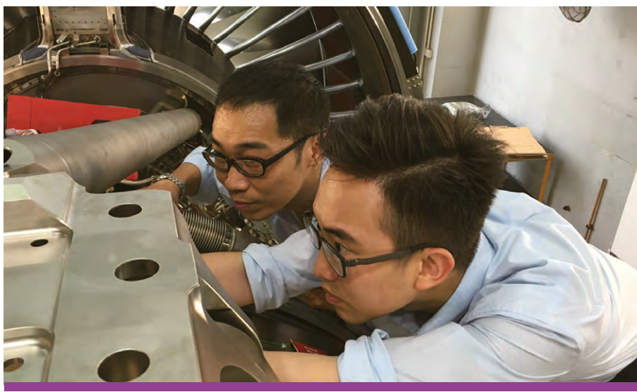
Module Change Engineers conducted the final inspection post installation of the Trent XWB engine mount.
