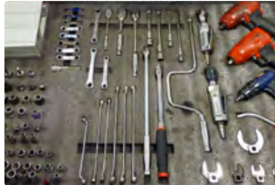
Example of Point-Of-Use Tooling at the HAESL work centre
