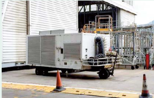
Previous Practice: Mobile diesel powered air-conditioning system
