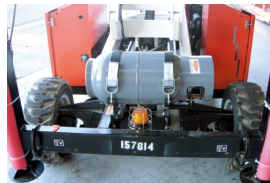
GSE with propane powered engine in HAECO Americas
