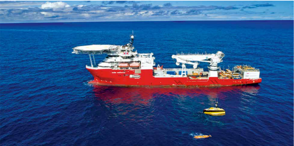
Seabed Constructor with a USV (unmanned surface vehicle – yellow vessel) and an AUV (orange submersible).
