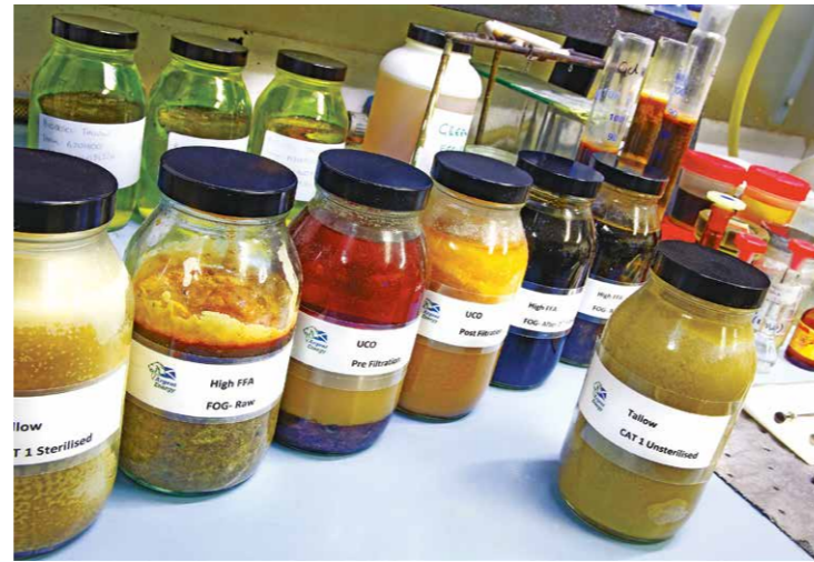
Argent Energy has pioneered a process that renders feedstock with a high Free Fatty Acid (FFA) content suitable for mainstream biodiesel production.
